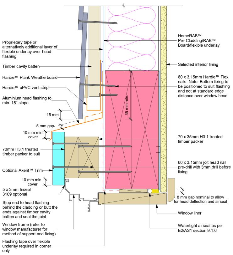
Note: Sealant must be installed between head flashing and window flange in VH and EH wind zones and SED pressures
